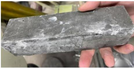
Fig.3 Image of Efflorescence.
